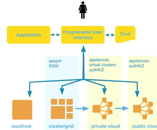
Figure 3 Simplified computational model of the infrastructure of the Swiss Compute Cloud project
